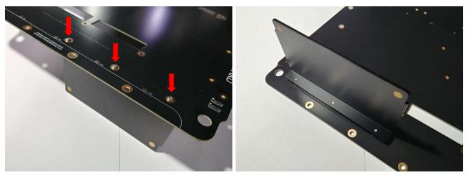
The PSU support bracket uses 2x #6-32 x 0.375" + 1x Nut. The Nut is only used if a short PSU is mounted, as this bracket uses the MB standoffs when a long PSU is used:
