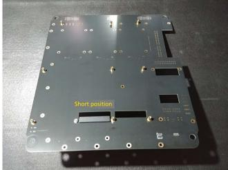
Motherboards are secured with  $9x #6-32 \times 0.25$ ".
