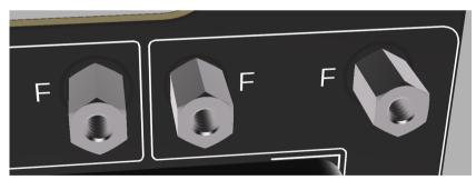
**Part B:** The remaining x4 of the #6-32 10mm SO-F female standoffs will have a #6-32 10mm SO-M male standoff on the opposing side instead of fasteners, these form the 4 mounting points for the ITX/DTX motherboard at the mounting holes marked with "M" on the front side of the main PowerBoard.
