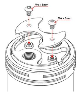
The ARGB Cover can be attached using the two included M4 x6mm Fasteners (see diagram beside).
