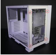
First remove the stock front glass panel from the case. Then the distribution plate can be installed in its place using the included M4 16mm Countersunk Fasteners, M4 Nuts and M4 Washers x4. The frame needs to be installed between the distribution plate and the case.
