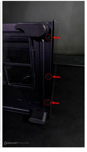
Once the front panel is removed the distribution plate can be installed in its place. Mount it from the front of the case. The Distribution Plate sandwiches the case panels on the bottom and on the right (the case panel goes in between the layers). The the x7 M4 10mm Fasteners can be tightened from the inside which will clamp the Distribution Plate onto the case panels.
