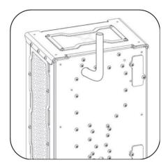
Arterial 2.0 Water-boxes have a dedicated fill and drain port. When filling it is best to connect a fill tube at least 20cm long. This is to prevent any overflow from back flow when the pump/s are turned off and helps to get the last of the air out. For draining a drain valve needs to be added to the drain port, or if you are using quick disconnects then the water-box could also be drained from those.
