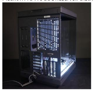
Mount the Distribution Plate to the rear panel fan mounting location. Move the Distribution Plate until the mounting holes are aligned with the slots on the case. Mount using the included M4 10mm Fasteners and M4 Washers (do not over tighten fasteners on acrylic). The distribution plate has some adjustment due to the slotted holes on the case, it is best to use this adjustment when installing the fittings. The included back plate can optionally be installed.
