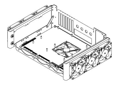
Install the motherboard using 9x M3 6mm BH fasteners. Install an ATX power supply using 4x #6-32 ¼" BH fasteners. Install PCIe cards and secure them using M3 6mm BH fasteners.
