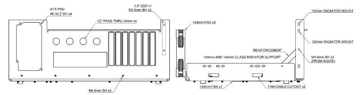
If radiators are going to be used in the system, install them now to the sides using the radiators' included mounting hardware. An offset fitting might need to be used with 280mm radiators to clear the power supply input cables and with 360mm radiators to make a connection to the D5 distribution plate (sold separately). There are cable routing holes on each side for the fans.
