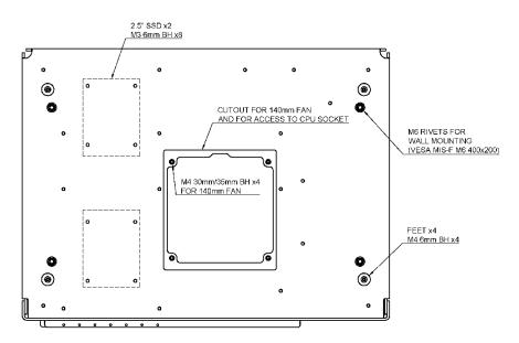
Install the back panel to the bottom panel using 5x M4 6mm BH fasteners, but do not tighten these fasteners for now. Install the reinforcement bars using 2x M4 6mm BH fasteners per bar driving the fasteners in from the inside, but do not tighten these fasteners either for now.
