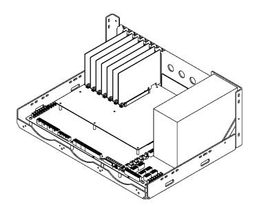
To the front of the case, we can attach up to 3x 140mm fans using M4 30mm BH for 25mm thick fans or M4 35mm BH fasteners for 30mm thick fans, or a D5 distribution plate using 6x M4 14mm BH fasteners. Graphics cards longer than 350mm interfere with the front fans and distribution plate.
