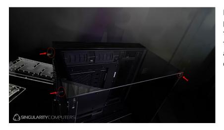
Remove the top panel and the side panel from the case. To remove the top panel the two thumbscrews on the rear panel need to be removed and the screw which holds the corner to the front panel.
