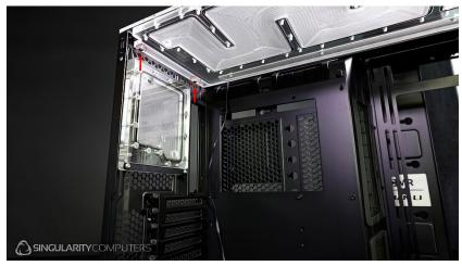
Also, x2 M4 10mm Fasteners need to be installed from underneath to clamp onto the rear panel of the case.
