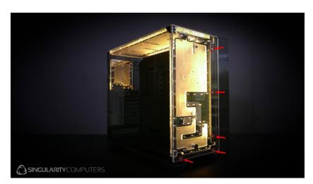
The Front Distribution Plate can then be attached to the case using x5 M4 12mm Countersunk Fasteners and M4 Nuts.
