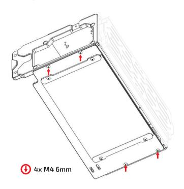
Attach the PSU Top Shroud (E) using M4 6mm x4. Attach the PSU Side Shroud (G) using M4 6mm x2 and M4 Stand Offs 10mm x2 at the bottom.
