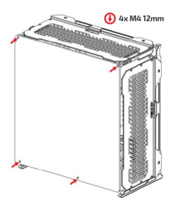
Install the Side Panel Window using 4x M4 12mm Fasteners.
