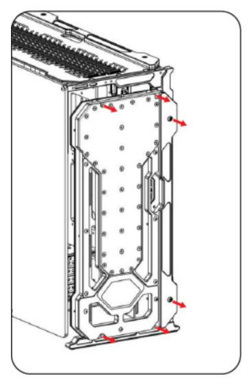
Spectre 4-M Elite comes fully assembled, remove the distribution plate from the radiator panel, then install the radiator, then the distribution plate can be reinstalled.
