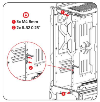
Attach the Rear I/O Panel to the case using 3x M4 8mm Fasteners.
