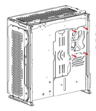
To install a rear 120mm fan, remove the rear cover by undoing the fasteners marked in the diagram. The Rear fan can then be attached to the back of the PowerBoard using M4 30mm x2 fasteners.
