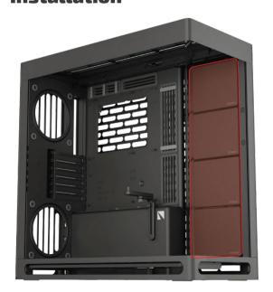
Remove the covers marked in the image. The HAVN HS 420 D5 Reservoir Combo Distribution Plate installs into this location using the included fasteners.
